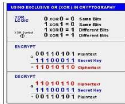
Keystream Generation Process in XOR Encryption System
